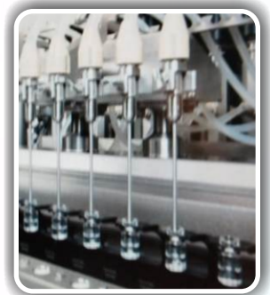
DOSING STATION WITH 12 WORKING POSITTONS
