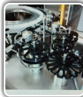
TRANSFER OF STERILIZED VIALS TO THE INDIVIDUAL TRANSPORT SYSTEM OF FILLING & CLOSING MACHINE
